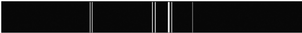
Figure 11.1. The spectrum of sodium (Kuhn's spectrum). From left red to right violet.
